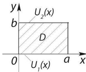
имеет вид  $u(x, y) = \sum_{n=1}^{\infty} \left[ \alpha_n \frac{\text{sh } \frac{n\pi(b-y)}{a} + b_n \text{sh } \frac{n\pi y}{a}}{\text{sh } \frac{n\pi b}{a}} \right] \sin \frac{n\pi x}{a}$ ,
